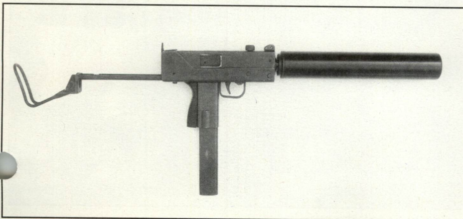
The R.A.S.E. SMG-45 suppressor dramatically outperforms other .45 ACP suppressors tested in this study.
