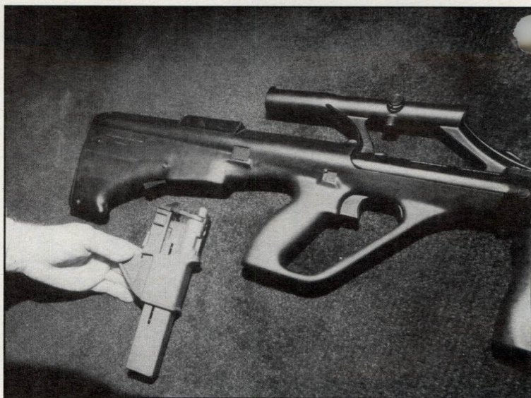
As you can see here, a change in the magazine well and a new magazine gets you on your way to converting your AUG to 9 mm. The barrel and bolt parts must also be changed but they are all currently available from Steyr.
